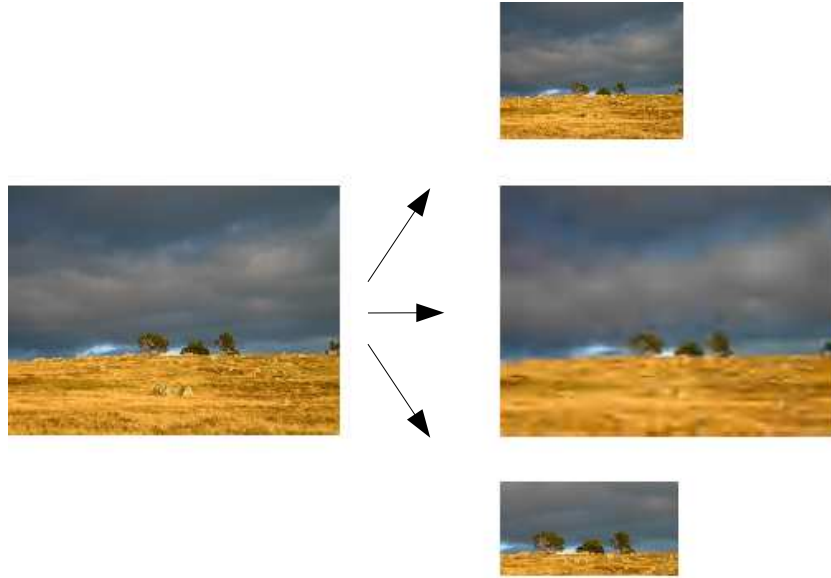
Figure 3.1: The image representation offers resolution (top), quality (middle) and spatial (low) scalability.
