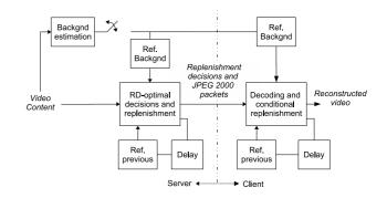
Fig. 1. Overview of the proposed JPEG 2000 video transmission architecture.
