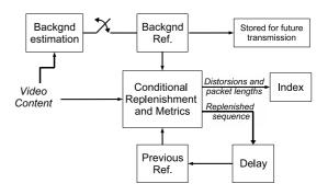
Fig. 3. Server off-line operations leading to the creation of the index.
