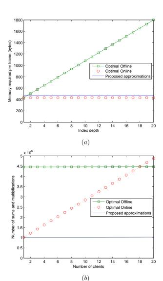
Fig. 5. Comparison of (a) memory and (b) computational resources for three different implementations of the proposed replenishment framework. Memory is depicted as a function of the index depth  $I_d$ , while computational resources are presented as a function of the number of server clients.
