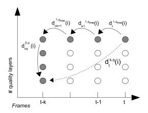
Fig. 4. Path used to approximate the distortion of the previous references, compared to the optimal path (dashed arrow). This approximation significantly decreases the pre-processing complexity and storage requirements, without significantly impairing the streaming performance.
