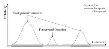
Fig. 6. Statistical modeling of a background pixel using three Gaussians. Multiple Gaussians aggregate the pixel luminance values observed in a sliding window.
