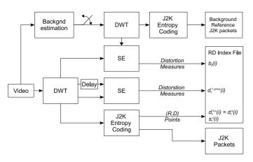
Fig. 3. Off-line operations leading to the creation of the RD index file at the server.
