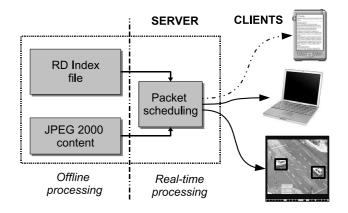
Fig. 1. Proposed video server architecture. Using a pre-calculated index, the server selects the optimal packets to transmit to each client, based on their individual needs and resources. Three types of clients are illustrated: a PDA client with a low resolution and low bandwidth, a laptop client with a high bandwidth and a third client focusing on two regions of interest for which he is expecting a high quality.
