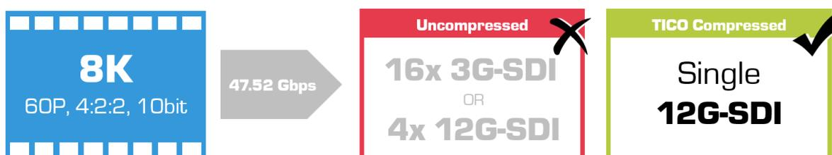
Deploying mezzanine compression for 8K not only saves cost, but also greatly reduces power consumption and infrastructure complexity. Next to a reduced amount of cables, TICO compression also reduces the amount of cross-points in a matrix switcher from 6400 to a mere 25.
